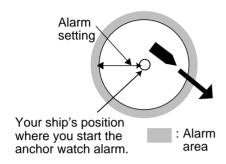
Figure 8-5 How the anchor watch alarm works
